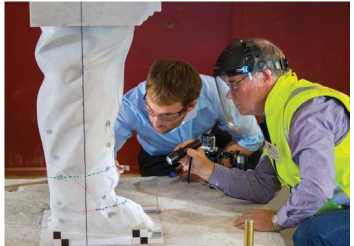
Engineers check the replica leg for cracking during the load testing process.
